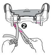
2. Pass the clip and the strap through the loop end  ${\rm \ensuremath{\mathfrak{O}}}$  as shown and pull strap up.
