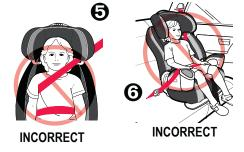
Vehicle seat headrest should not create a gap between vehicle seat and booster seat **O**. The front of booster seat **MUST NOT** hang over front of vehicle seat **O**.
