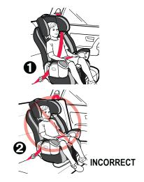
**DO NOT** use shoulder belt loose or positioned under arm  $\boldsymbol{\Theta}$ .
