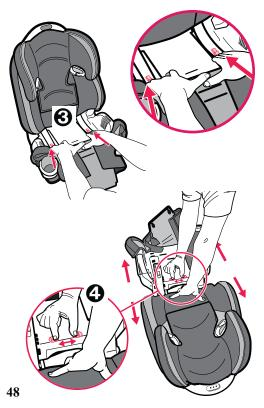
5. Once back support is separated **③**, store back support with all the harness straps, head support, body support and crotch pad cover in safe place.
